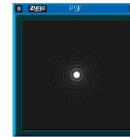
Airy disc of reference system w/o film, Strehl ratio 99,9%
