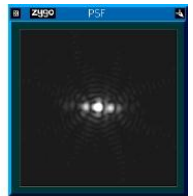
Airy disc with Mylar™ Strehl ratio 57,2%
