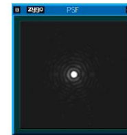
Airy disc with TurboFilm™ Strehl ratio 96,8%
